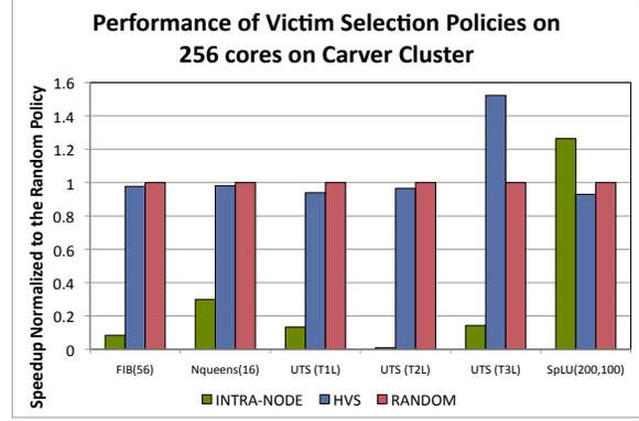
**Figure 10.** Performance comparison of stealing strategies on distributed memory: 256 cores on the Carver IBM iDataPlex cluster. The speedup numbers are normalized to the speedup of the random policy.
