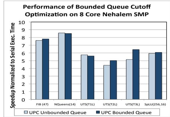
**Figure 8.** Performance comparison between HotSLAW with unbounded (UPC Unbounded Queue) and bounded queues (UPC Bounded Queue). Both UPC versions are optimized with tree-depth cutoff optimization. Experiments are run on a 8 core Nehalem SMP.
