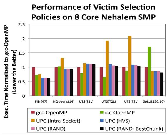
**Figure 9.** Performance of OpenMP and victim selection strategies on a 8 core Nehalem SMP. Execution times are normalized to the execution time of the gcc-OpenMP version (lower the better). All UPC versions use a fixed chunk size of 1, except the UPC (RANDOM+BestChunk) uses the best chunk size searched. For reference, the raw speedup numbers of UPC (HVS) scheme for (FIB, NQueens, UTS(T1L), UTS(T2L), UTS(T3L), SparseLU) are (7.7, 7.9, 7.5, 7.2, 7.5, 5.9), respectively.
