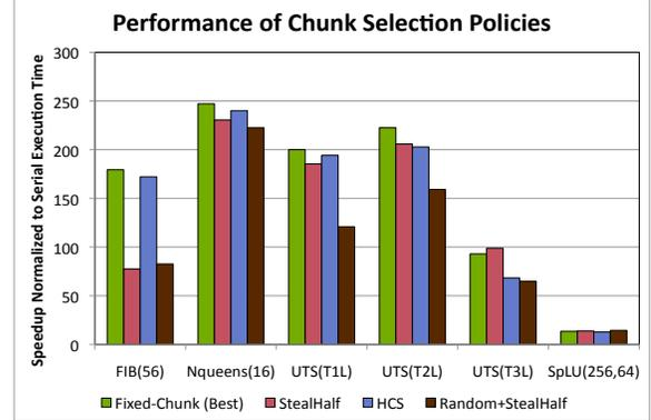
**Figure 13.** Performance of different chunk size selection policies on 256 cores Carver. *Fixed-Chunk (Best)* uses the best chunk size for each application and *HCS* uses a chunk of size one for its intra-node stealing. *Fixed-Chunk (Best)*, *StealHalf*, and *HCS* use *HVS* for its victim selection, while *Random+StealHalf* uses random victim selection.
